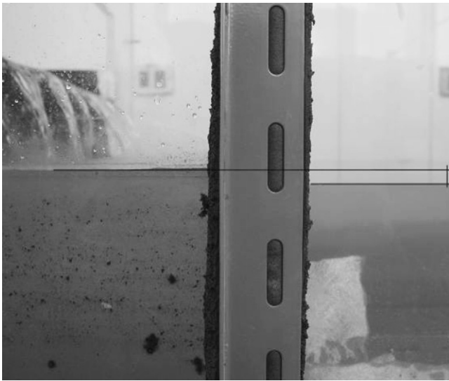
Fig. 3. Water level difference between the zone of the hydraulic plug and the zone over the filter system of the SCPT.
